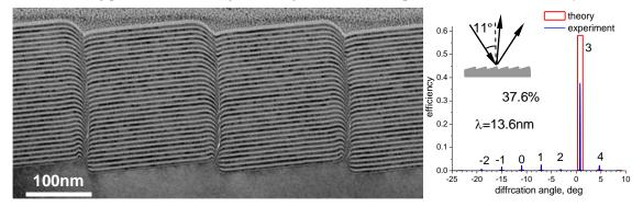
**Figure 2.** Cross-section TEM image of a MBG with groove density of 5000 lines/mm and the blaze angle of 6°, coated with a Mo/Si multilayer (left). Diffraction from the grating at the wavelength of 13.6 nm and the incident angle of 11° (right).
