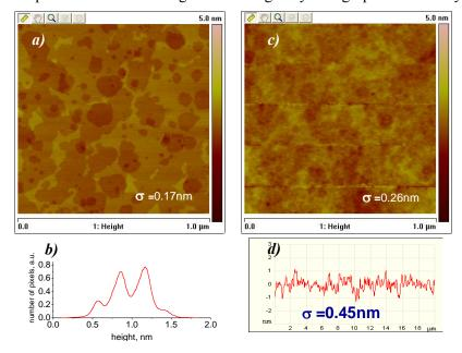
**Figure 1.** An AFM image of a  $1 \times 1 \ \mu m^2$  area of anisotropically etched (111) surface of Si (a) and a height distribution in the same area (b); an AFM image of a  $1 \times 1 \ \mu m$  area of a saw-tooth substrate with an average groove profile subtracted shows residual high frequency roughness (c), and a 20 \ \mu m long AFM scan along a groove of a sawtooth substrate shows midfrequency roughness (d).
