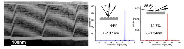
**Figure 3.** Cross-sectional TEM image of a MBG with groove density of 5250 lines/mm and a blaze angle of 2°, coated with a Mo/Si multilayer (left). Diffraction from the grating at the wavelength of 13.1 nm and an incident angle of 7° (center), and 1.34 nm and 85.5° (right).
