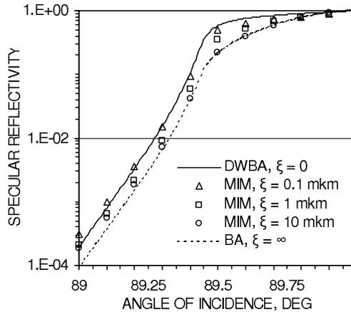
Figure 5: Specular TE reflectance of Au mirrors calculated for  $\sigma = 1.5$  nm and different  $\zeta$  for  $\lambda = 0.154$  nm vs. angle of incidence.
