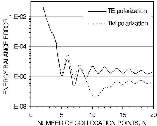
Figure 1: Using the *SIM* for the problem of diffraction on a plane interface for  $\lambda/d = 1$  (normal incidence,  $n_0 = 1$ ,  $n_1 = 1.5$ ).
