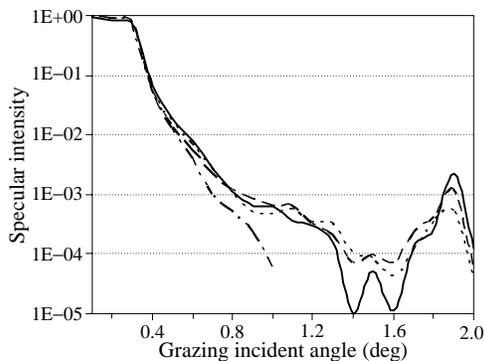
**Fig. 1.** Absolute specular reflectivity for sample F668 with vertically non-correlated GDs at a 0.154-nm wavelength vs grazing angle of incidence: perfect plane structure model (short-dashed line); Névo-Croce approximation with rms roughness of 1.45 nm for triangles (long-dashed line); rigorous calculation with QD height  $h = 5$  nm and width  $L = 16.7$  nm (full line); measurement (long-short-dashed line).
