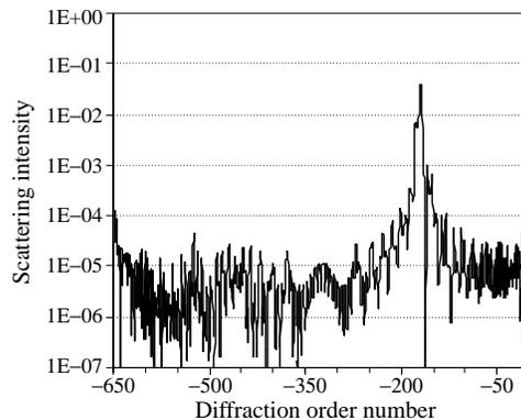
**Fig. 2.** Absolute specular and non-specular reflectivity calculated for sample F667 with vertically correlated GDs at a 0.154-nm wavelength and a  $0.5^\circ$  grazing incidence vs diffraction angle in the range from  $-85.7^\circ$  to  $+89.7^\circ$ . The strong peak exists near a scattering angle of  $28.5^\circ$  that corresponds to specular reflection from QD facets.
