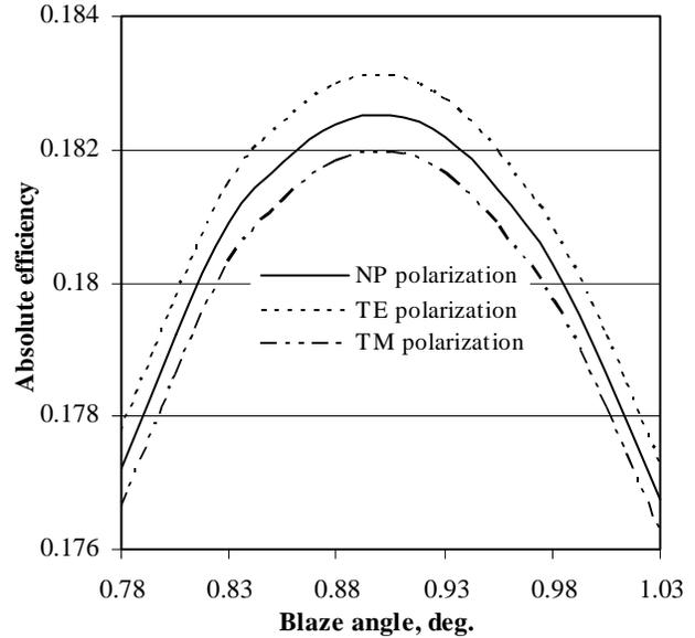
Fig. 3. Absolute  $-1$  order efficiency of a 1000-gr/mm sawtooth grating with  $0.9^\circ$  blaze angle and  $10\text{-}\text{\AA}$  rms roughness calculated for a  $15\text{-}\text{\AA}$  wavelength as a function of polar incidence angle for the in-plane mounting.
