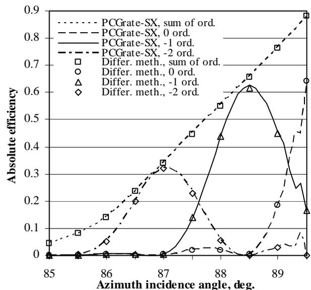
Fig. 2. Absolute efficiency in the 0, -1, and -2 orders of a 3600-gr/mm sawtooth grating with 5° blaze angle calculated for a 13.34-Å wavelength incident at 5° polar angle as a function of azimuth incidence angle for the off-plane mounting.
