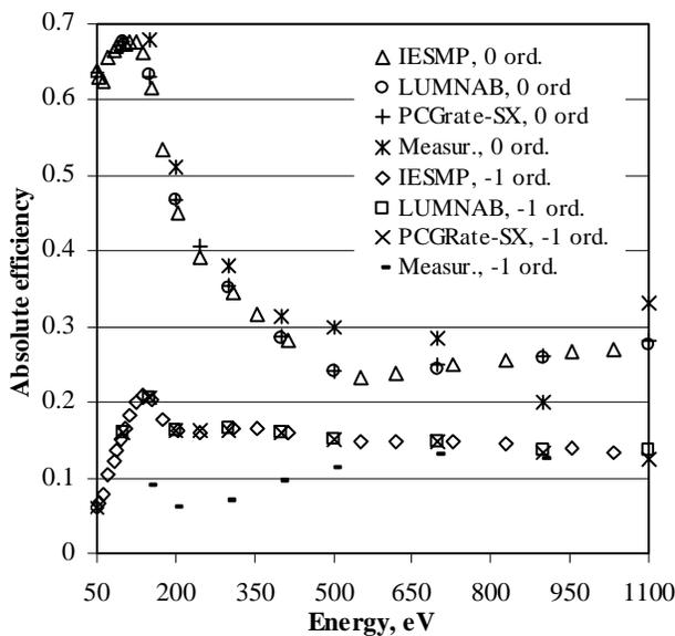
Fig. 1. Absolute efficiency in the 0 and -1 orders of a 1200-gr/mm sawtooth grating with 1.3° blaze angle and 2.25 fixfocus plotted as a function of energy for the in-plane mounting.
