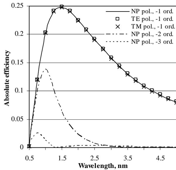
Fig. 6. Absolute efficiency in the  $-1$ ,  $-2$ , and  $-3$  orders of a 641-gr/mm sawtooth grating with  $0.75^\circ$  blaze angle and  $10\text{-\AA}$  rms roughness calculated as a function of wavelength at the  $88.43^\circ$  polar incidence angle and the in-plane mounting.
