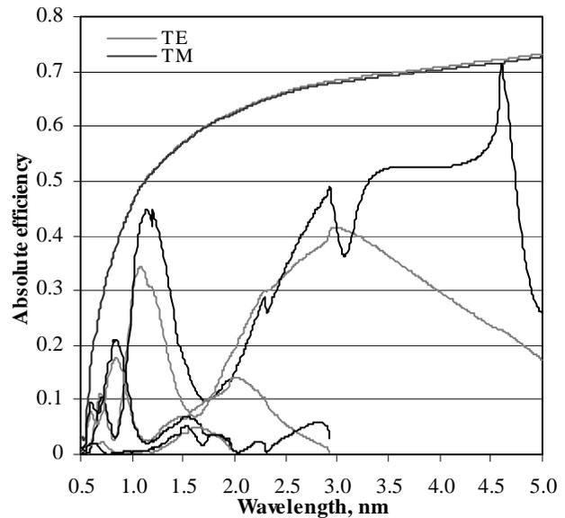
Fig. 13. Same as in Fig. 8, but for a polygonal grating with rms roughness of  $20 \text{ \AA}$  and an azimuth incidence angle of  $88.5^\circ$ .
