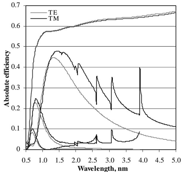
Fig. 8. Absolute efficiency in the  $-1$ ,  $-2$ , and  $-3$  orders of a 5000-gr/mm triangular grating with  $7^\circ$  working facet angle and  $5\text{-}\text{\AA}$  rms roughness calculated as a function of wavelength for the  $7^\circ$  polar and  $88^\circ$  azimuth incidence angles and the off-plane mounting.
