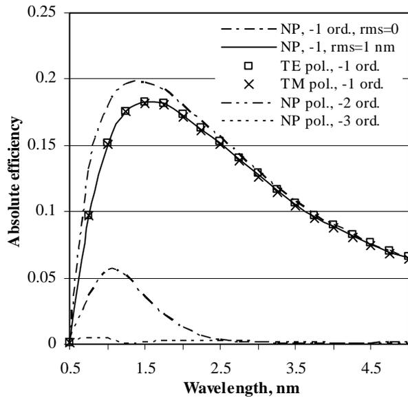
Fig. 5. Absolute efficiency in the  $-1$ ,  $-2$ , and  $-3$  orders of a 1000-gr/mm sawtooth grating with  $0.9^\circ$  blaze angle calculated as a function of wavelength for the  $88.1^\circ$  polar incidence angle and the in-plane mounting.
