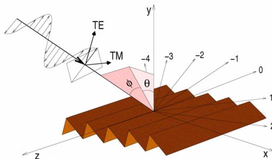
Figure 1: Schematic conical diffraction by a grating.
